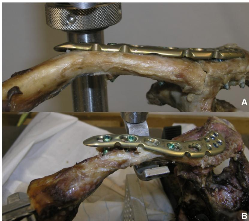
Fig. 4. Modes of failure of the single-plate technique. A) fracture adjacent to the innermost screw (9/10), B) pull out of the two most medial screws (1/10).
