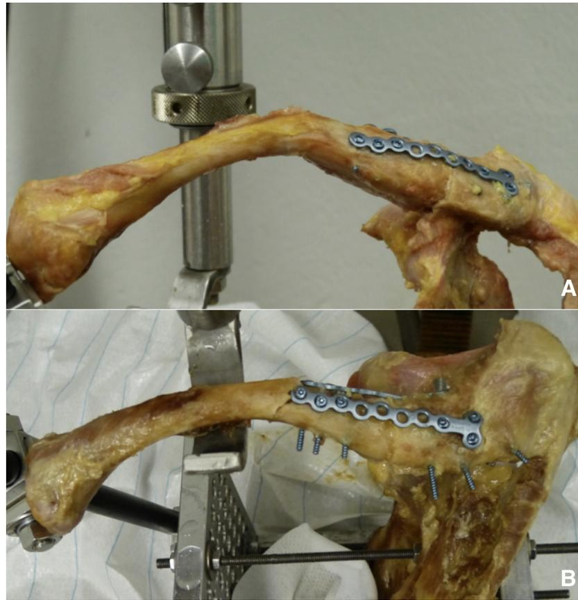
**Fig. 5.** Most frequent modes of failure of the double-plate technique. A) fracture adjacent to the traction device position (4/10), B) fracture adjacent to the innermost screw (3/10).
